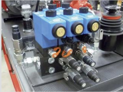
Block CETOP 3 function for on-off controls
