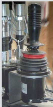
3-Axis proportional manipulation for PVG 32 control
