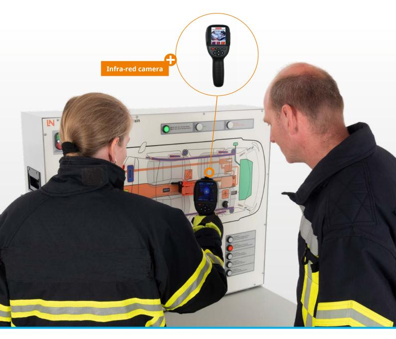
Thermal imaging is a safe and effective method of assessing the fire hazard potential of a high voltage vehicle involved in an accident. If there is any suspicion that the integrity of the high voltage battery is damaged, the temperature should be analysed as quickly as possible and continue to be monitored.
