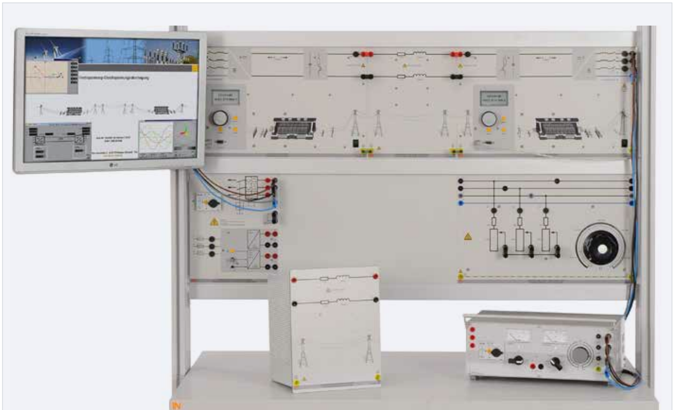
Experiment example "High voltage DC transmission" EDC1
