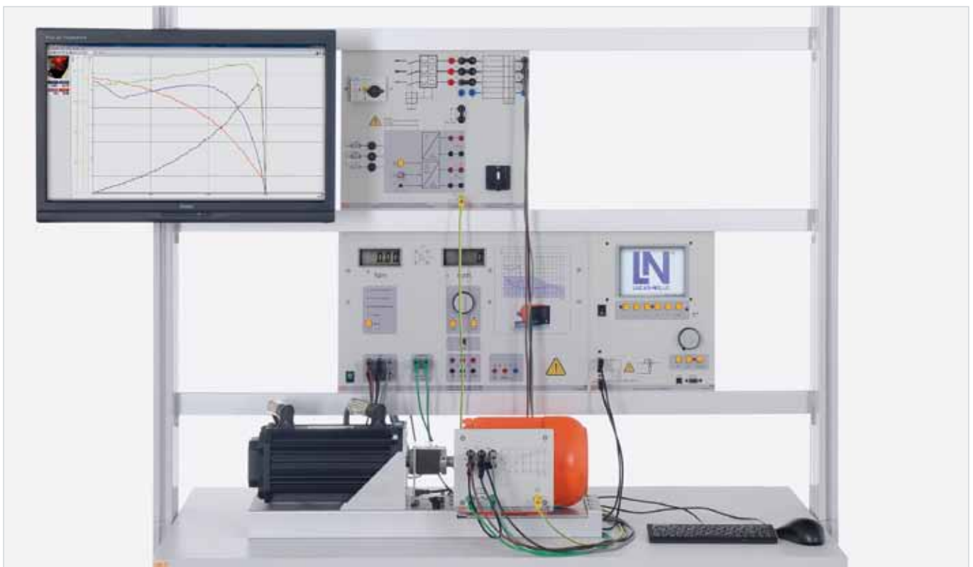
The "Energy-saving motors" training system consists of a highly efficient motor and a servo machine test stand.
