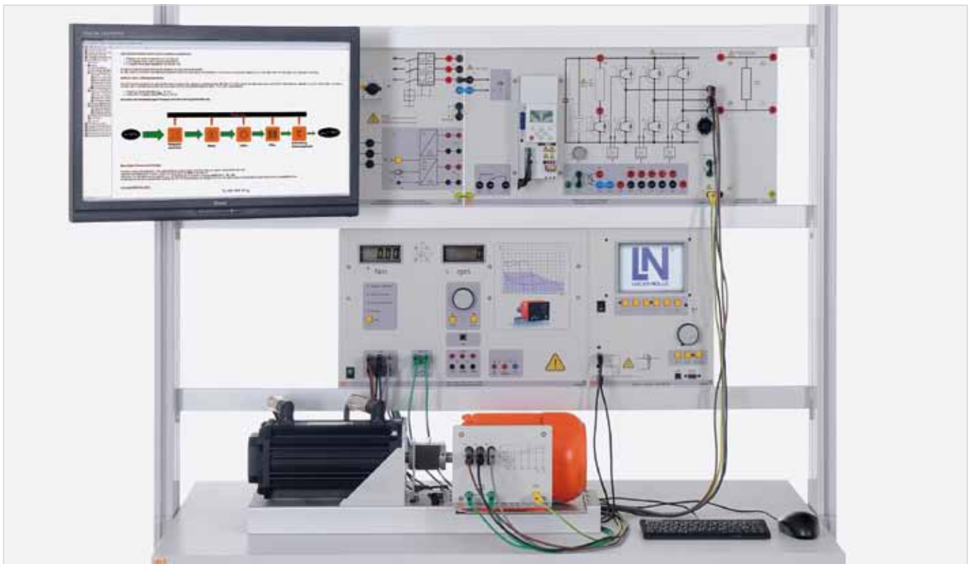
The "Energy-efficient drives with frequency converters" training system consists of a highly efficient motor, frequency converter and servo machine test stand.
