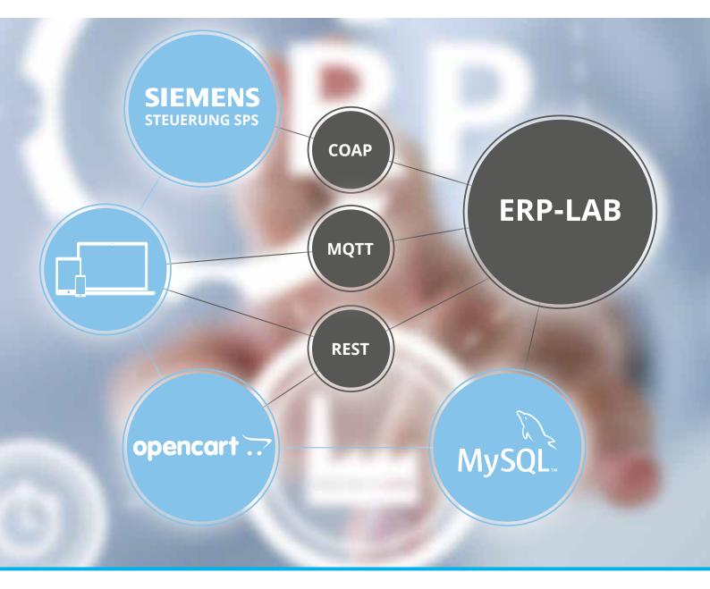
In its function as a **Manufacturing Execution System** (MES) the ERP Lab monitors the entire process. As a server-based system it provides all production-relevant data within the Edge Cloud (Cloud services in the intranet) – ranging from the Webshop to the production process all the way to warehousing. The system also communicates with the programmable logic controls of the production line via the network.
