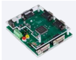
FPGA Altera Cyclone IV
