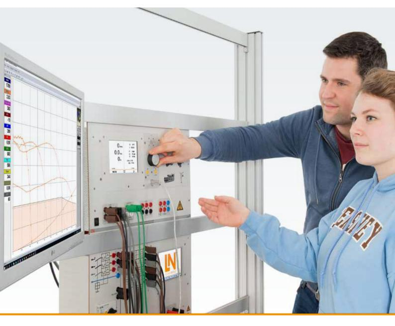
Various programs specialized for specific needs permit the servo machine test system to be operated via the PC.
