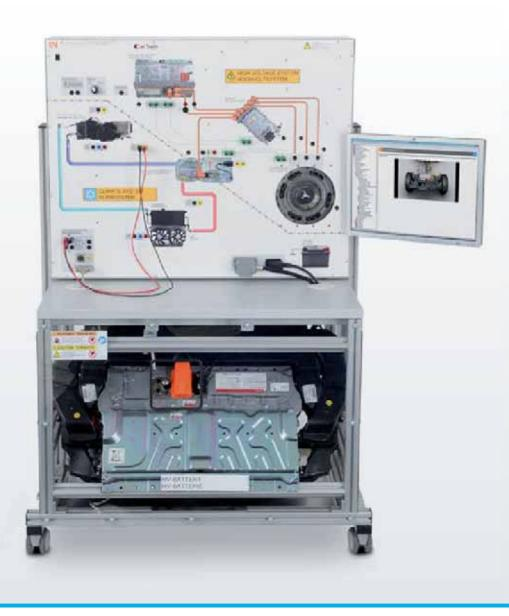
Combined equipment for the topics of hybrid drive trains and high voltage air conditioning in vehicles. Trainees can use the set to learn about the aspects of servicing, diagnostics and repair of high-voltage networks and air conditioning.
