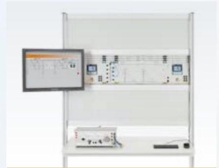
EUL 3 – Transmission line with earth fault compensation
