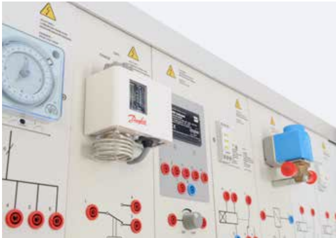
Authentic components from refrigerators and special compressor starting circuits, such as those using part-winding motors, ensure an insight into typical refrigeration circuits much like those used for refrigerators in practice.
