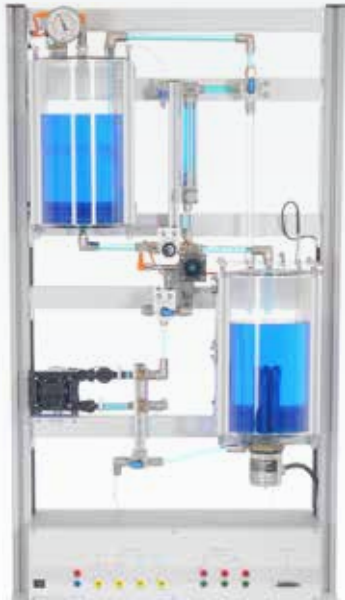
Process Engineering Compact Station with digital controller
