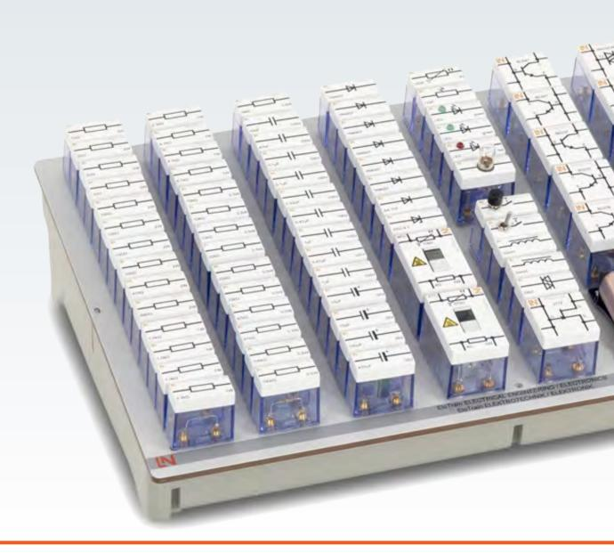
With this equipment set consisting of 82 individual 4-mm plug-in modules, a multitude of electrical engineering and electronics experiments can be set up. In addition to the experiments covered in the "DC technology", "AC and three-phase technology", "Semiconductor elements" and "Basic circuits in electronics" manuals, a vast array of additional circuitry can also be implemented. The set is delivered on a DIN A3 storage board with scratch-proof, coloured imprint.
