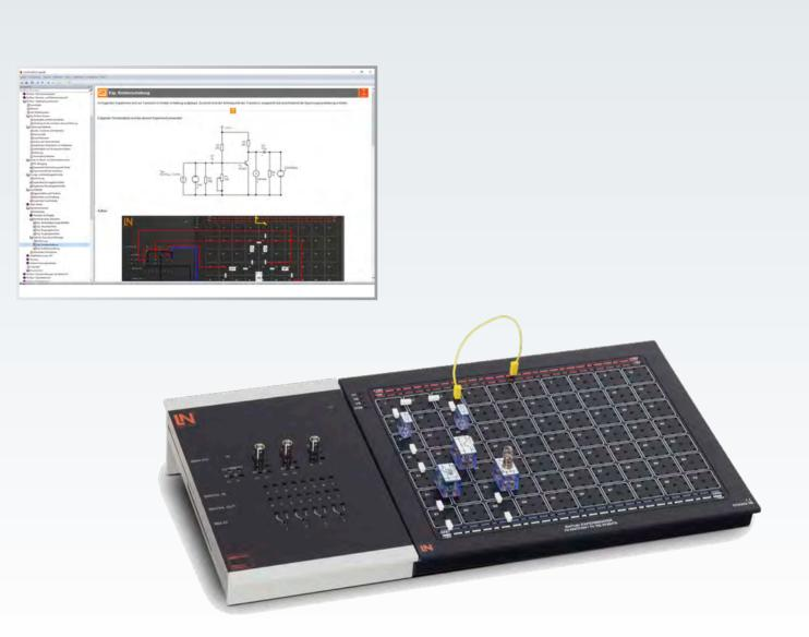
Knowing the properties and functions of electronic components is fundamental to an understanding and analysis of electronic circuits and ICs.
